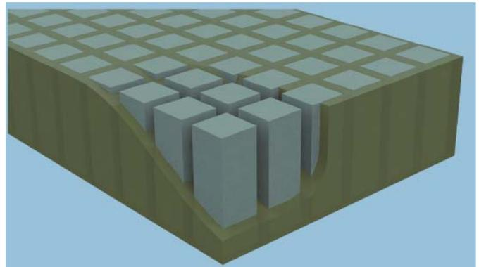
**Figure 1 - In composite transducers, the transduction is performed by individual ceramic staffs that are free to move independently of each other.**
